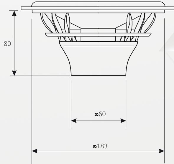
Alle Maße in Millimeter | All dimensions in millimeters
