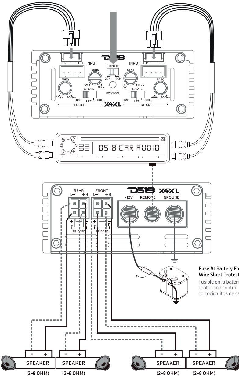
Fuse At Battery For Wire Short Protection
