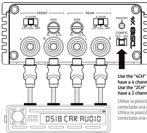
Use the "4CH" position when you have a 4 channel RCA input connected
