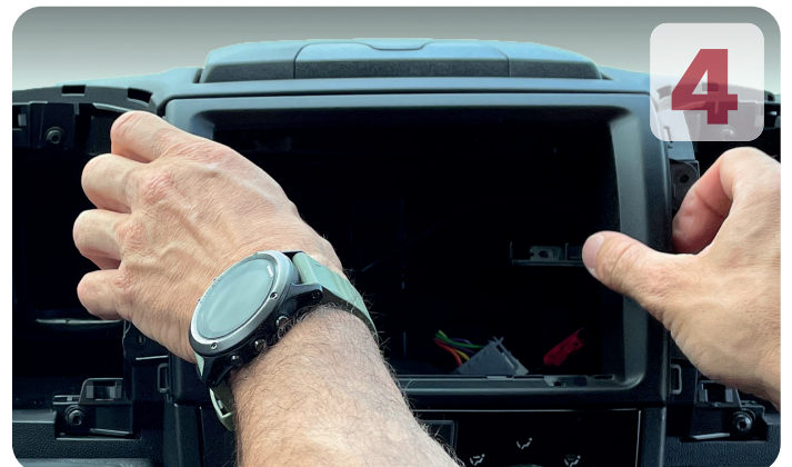
Remove the original frame from the dashboard
