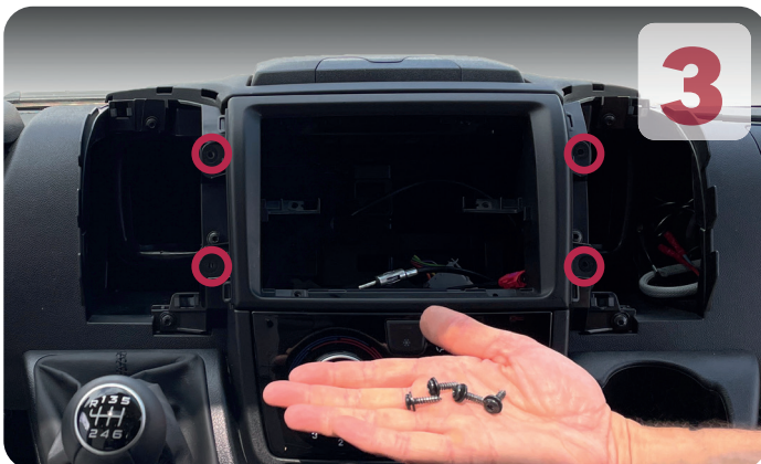
Remove four screws using a T20 screwdriver Keep them a side for later
