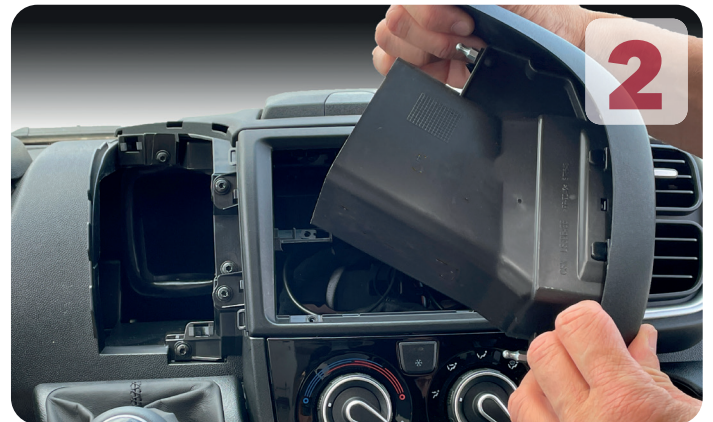
Remove the airvents left an right by pulling They are attached with two pins
