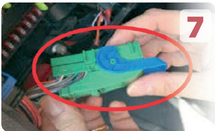
Open the green connector and slide the cables out
