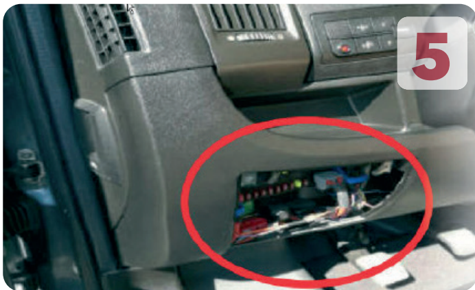
Open the fusebox underneath the steering column
