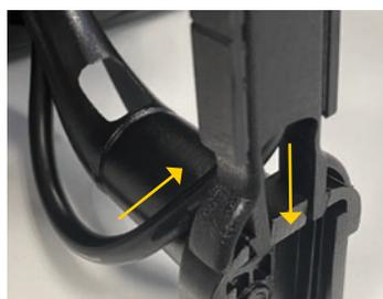
Using the included cable channel, the monitor's connection cable can be routed discreetly to the roof lining.
