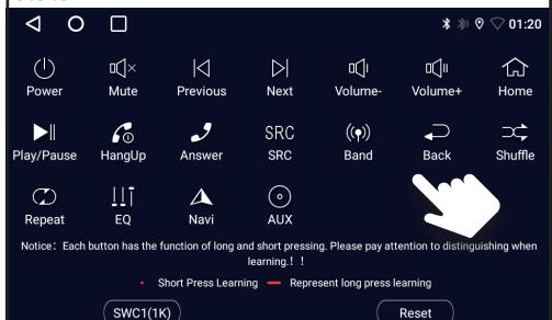
**N.B. Every control on the steering wheel can respond to either a short or long press.**
