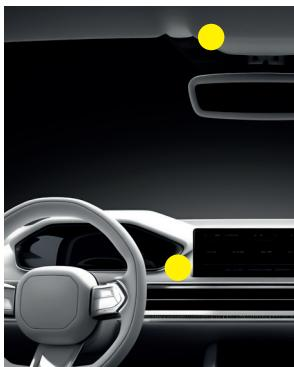
Find the best spot to place the microphone (7) inside the vehicle, making sure it faces and is near the driver for optimum performance. Attach the support with 3M double-sided adhesive tape.
