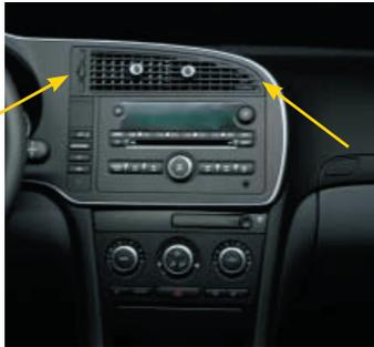
Gently remove the air ventilation shaft with a plastic wedge.
