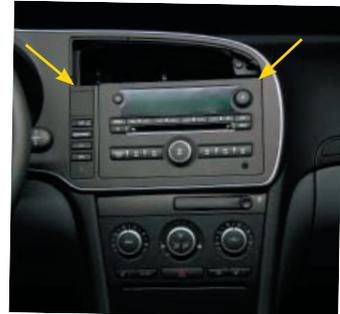
Remove the torx screws at the location of the arrows and remove the radio.
