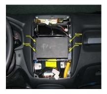
Use plastic wedge to remove panel and remove 4 screws.
