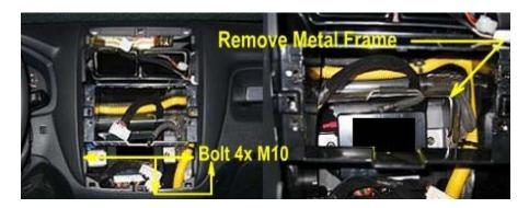
Remove 4x M10 bolt and remove Metal Frame complete.
