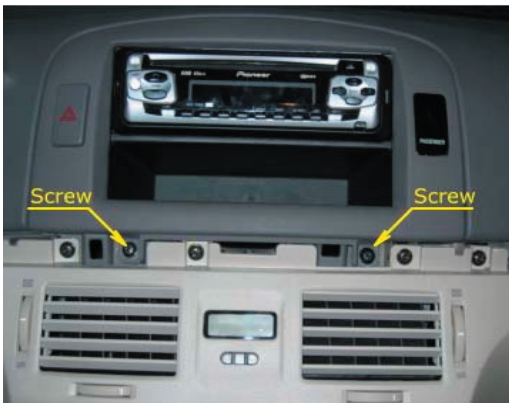
Remove 2 screws and use plastic wedge to remove panel.
