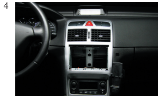
Place the 2-Din metal bracket.
